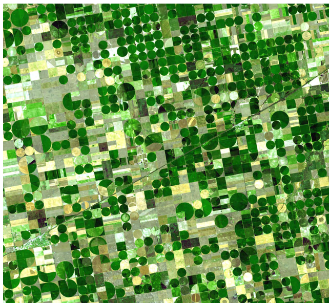
A 2001 satellite image of farms in southwestern Kansas illustrates the green circles that center-pivot irrigation systems produce. The unirrigated areas outside the circles are potentially available for solar PV installation.
