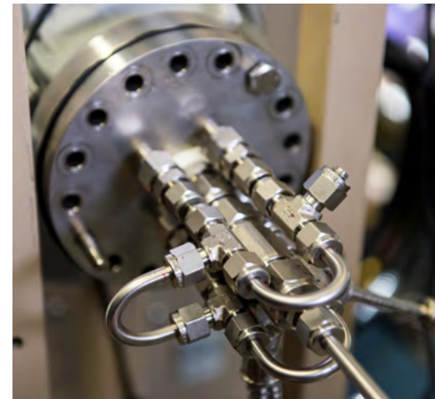
Developing components suitable for transporting and burning hydrogen is key challenge for utility-scale hydrogen power systems. Pacific Northwest National Laboratory uses the MTI Hydrogen Furnace to test how hydrogen affects various materials.
